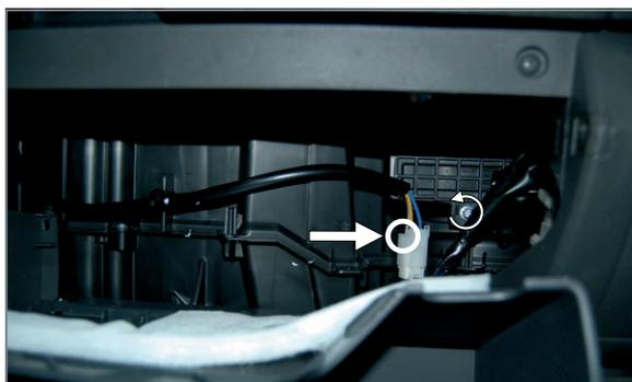
(EN) Disconnect the electric circuit. Open the filter chamber
